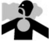
**WARNING: NEVER** run the engine in an enclosed area. Exhaust gas contains carbon monoxide, an odorless and potentially deadly gas.
